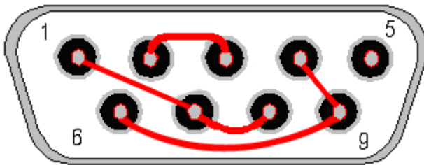
Female DB-9 connector - Rear view
